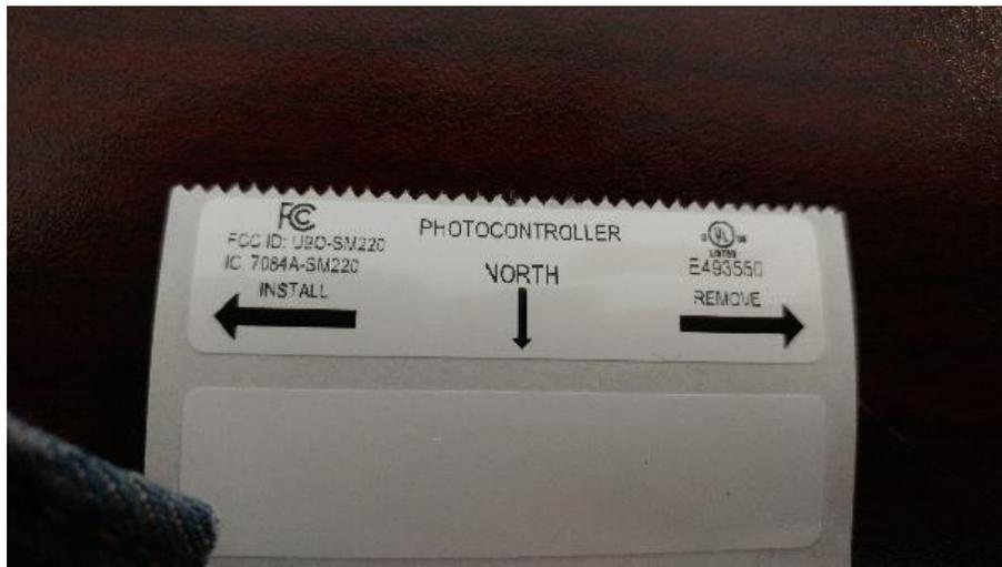
**NOTE: Align 'North Arrow' on label with North Arrow on base as shown below – LABEL SHOWN IN IMAGE BELOW IS FOR REFERENCE ONLY, USE REQUIREMENTS NOTED ABOVE FOR LABEL PRINTING.**
