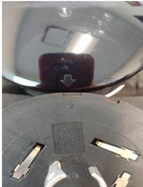
Set cover/base assembly onto the arbor press tool and gently press cover onto base as referenced in the video.
